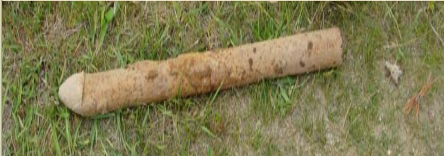
The aircraft rocket is approximately 29 inches in length and 2.25 inches in diameter.
