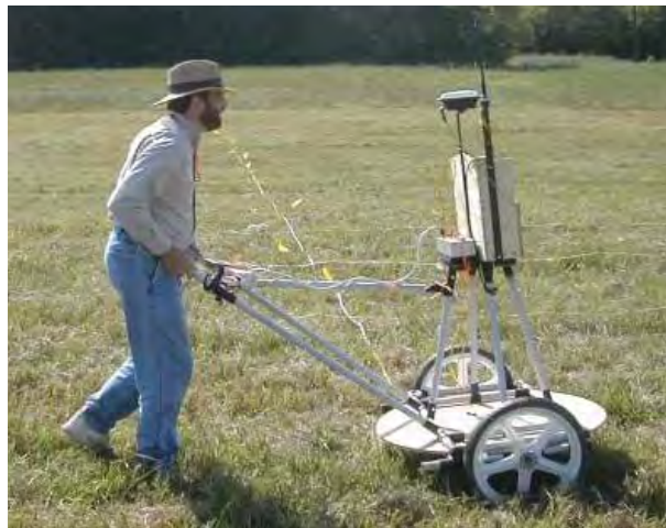
Figure 6. The GEM-3-E during survey.
