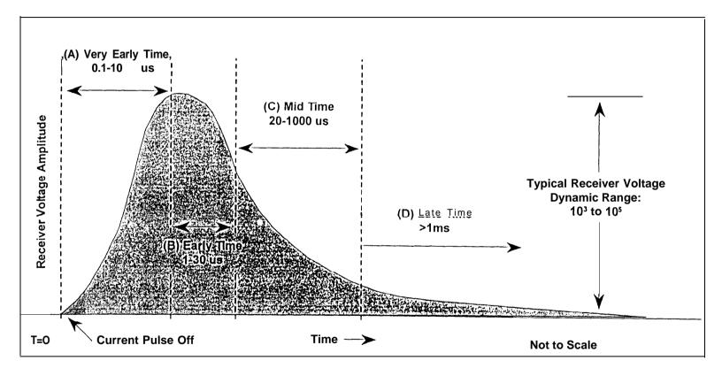
A. Very Early Time: Currents form in target conductor to preserve the original magnetic field before turn-off.
