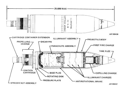
*Use.* This cartridge is used for target and battlefield illumination at night and during other periods of low visibility.
