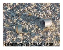
These are just a few examples of the types of discernible scrap / debris that are left over by design. It would seem as though a study or characterization on what was "expected" to be on a range would be beneficial as then you could eliminate these types of targets from your list as they present little to no hazard compared to a high explosive UXO. In essence, sometimes in order to find what you are looking for, you must first understand what you are not looking for.
