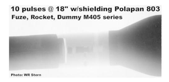
Though having identical external features, x-rays of 3.5-inch rocket fuzes illustrate the distinguishable internal difference between the M404 series fuzes and M405 series fuzes. Matching the x-rays with drawings for the M404 and M405 in the applicable publication removes all doubt which fuze is present.
