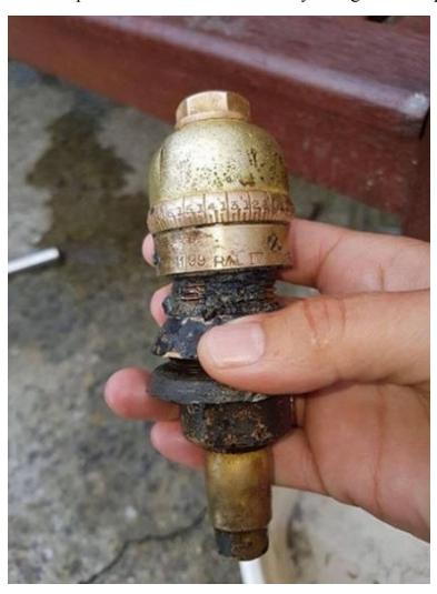
EOD identified the fuze as that of a WWI shrapnel projectile, anti-personnel artillery munition. The remainder of the shell had corroded away over the years, leaving just the fuze and scattered debris.
