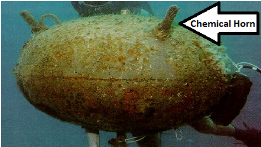
Chemical horns are the firing mechanisms on a sea mine
