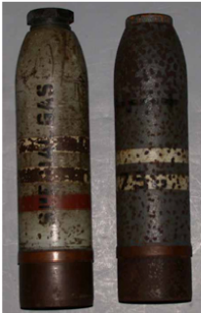
WW I CWN shell (Note the hex plug on ogive):
