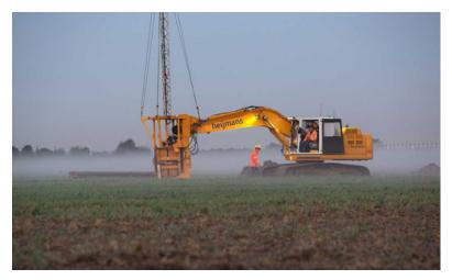
For the mock German airfield site, a grid size was 2.5 meters by 2.5 meters was selected for the magnetometer probing with the maximum average depth of each probe reading ranging between 8 to 10 meters or until the probes reached a sand layer with a density less than 10 MPa.
