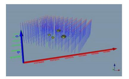
The 3D map of the UXOs is also a useful tool for the recovery team as they have an accurate map of the locations of targets which need to be investigated including information on size and depths of targets. To date, 40 bombs have been cleared from the site including a variety of German bombs ranging from the SC-50 (50 kg) to SC-500 (500 kg) bombs.
