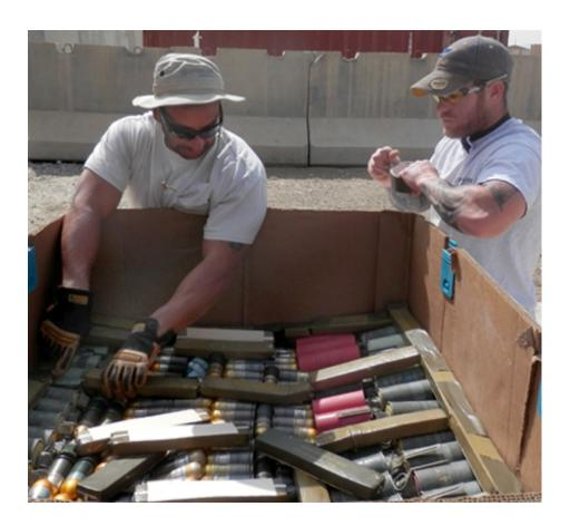
Joint Munitions Disposal-Afghanistan personnel build an ammunition shot box and place C-4 over the unserviceable ammo scheduled to be destroyed, paying particular attention to the continuity of the explosives and ammo. It is then taped in place for extra security from movement to the range for demolition.
