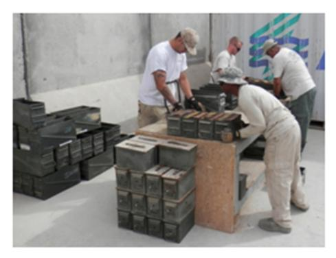
Personnel supporting joint munitions disposal operations in Afghanistan are delinking .50 caliber rounds, or taking them out of their links, and placing them loosely in cans for later burning in the
