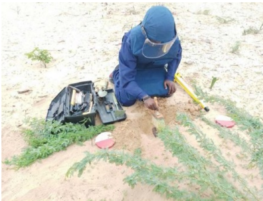
Figure 3 - Searcher excavating ERW detected on the spot using Schonstedt UXO Locator (Magnetic Locator) in Daynile, Somalia.
