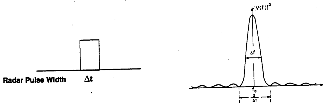
Figure 2.2.3.2. Transmitted radar pulse width and system bandwidth.
