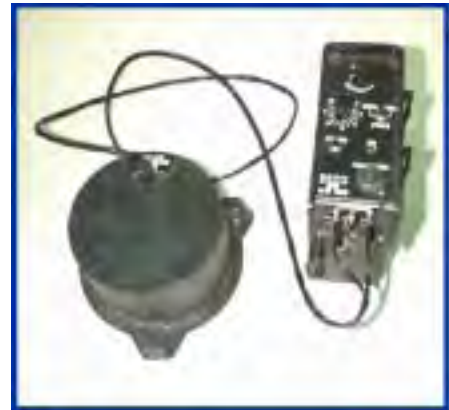
DIGS search head and electronics unit. The search head clips into the AN/PSS-12 metal detector.
