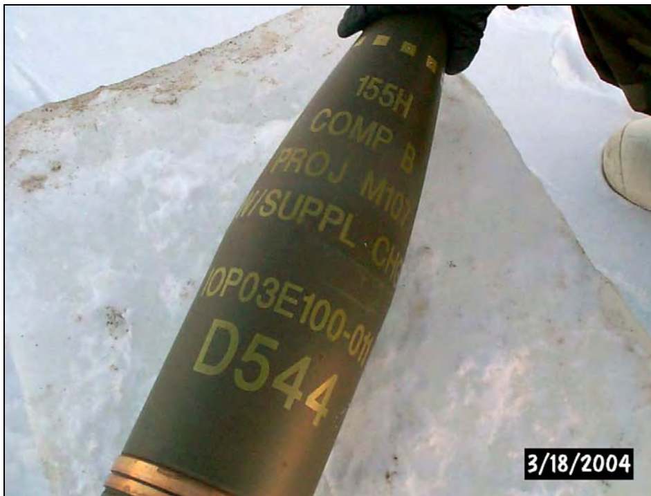
Figure 2. 155-mm projectile used in baseline and alternative BIP tests.
