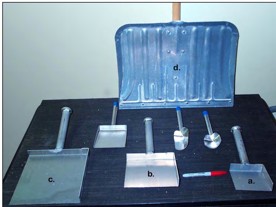
Figure 4. Snow sampling tools. a. 10- × 10- × 2-cm scoop; b. 15- × 15- × 2-cm scoop; c. 20- × 20- × 2-cm scoop; d. 45-cm snow shovel (original sampling method).
