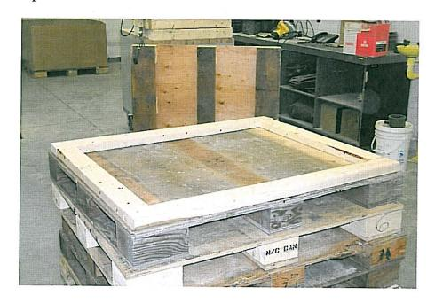
iii. Using ¾ inch 4" X 8" plywood, cut to fit and place along the sides of pallet. Secure.
