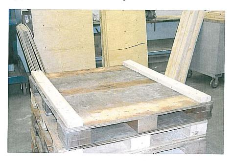
ii. Place qty 2 2" X 4" on the inner ends of the pallet, again leaving enough space to place a piece of plywood flush with the side of the pallet. Secure.
