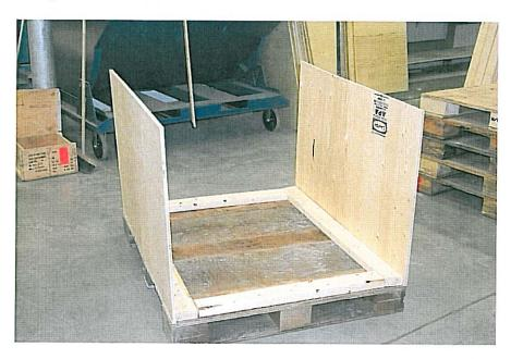
iv. Using ¾ inch 4" X 8" plywood, cut to fit and place along the front and back of pallet. Secure.
