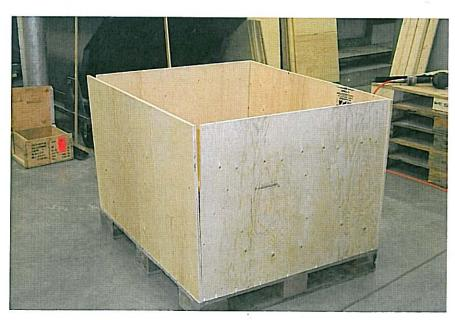
v. Using 4" X 4" posts, cut to fit from bottom of pallet to flush with top of plywood. This will allow for the 4" X 4" to support the triwalls during stacking. Secure.
