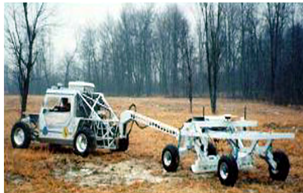
Multi-Sensor Towed Array Detection System is an example of the newer generation of vehicle towed systems.
