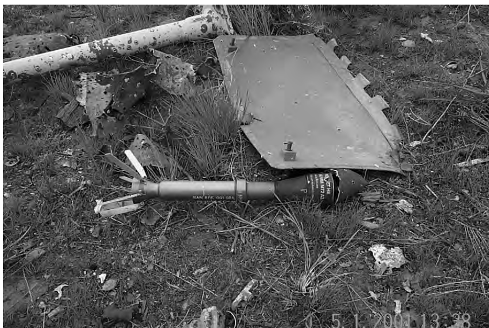
Figure 4. Ruptured LAW Rocket at Yakima Antitank Range
