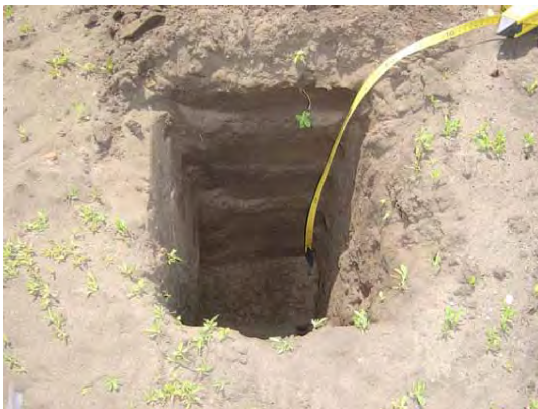
Figure 4-10. Vertical sampling in one of two holes 60-cm deep at firing point in Range 22.
