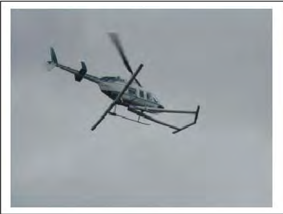
Figure 9-3 Airborne Geophysical Survey Helicopter Platform (from ORNL, 2002).
