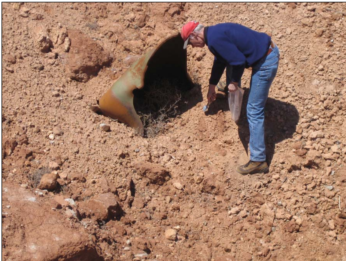
Figure 12. Soil sampling being conducted near a low-order 2000-lb bomb at Holloman Air Force Base, New Mexico.
