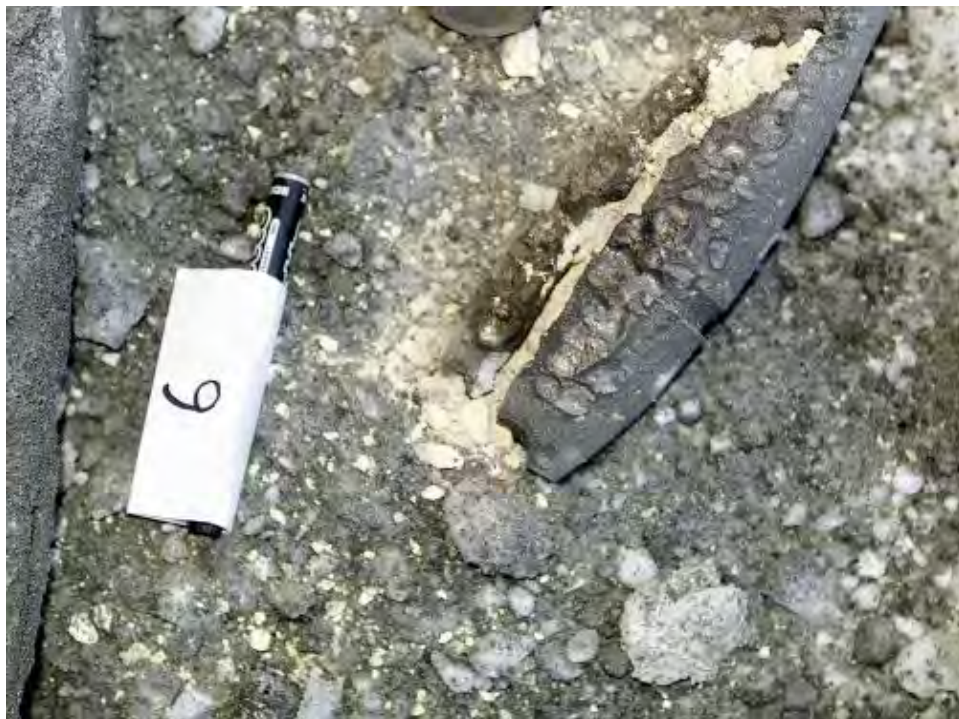
Figure 7-6. Projectile attacked by fragments at a short distance (Trial #6)
