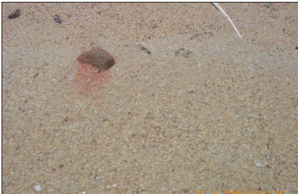
Figure 10. Small chunk of explosive showing halo of color that develops as these chunks weather, found at the Emerson Lake Range, 29 Palms, California.
