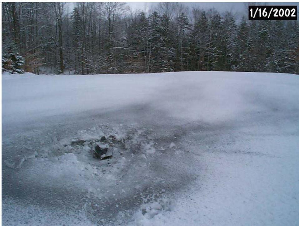
Figure 6. Post-blast residue of a C4 block with M6 blasting cap at Camp Ethan Allen, Vermont. A metal plate was placed under the snow to minimize disturbance of the underlying soil.
