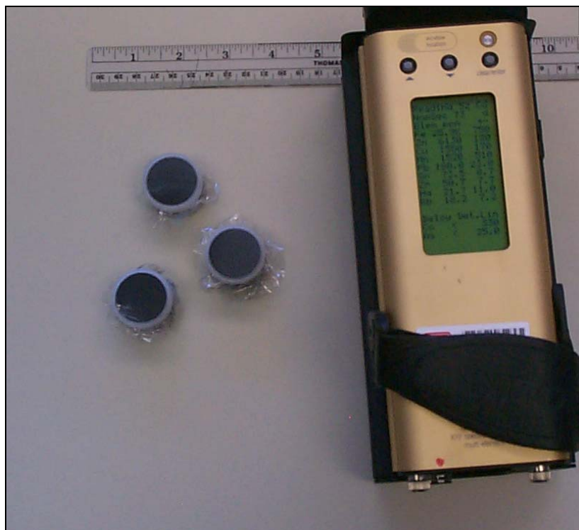
Figure 2. FP-XRF analyzer used in this study. On the left are samples of post-blast residue contained within XRF sample cups.
