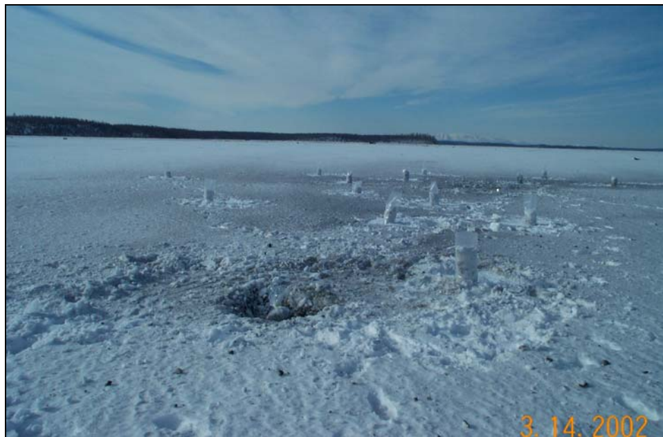
Figure 1. Post-blast residue plume from a 105-mm howitzer projectile. Samples of the solid residue were collected by shoveling darkened snow into bags, melting the snow, then filtering the meltwater. (Photo courtesy of Michael R. Walsh.)
