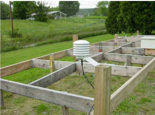
Figure 2. Test frame for frost-jacking experiment.
