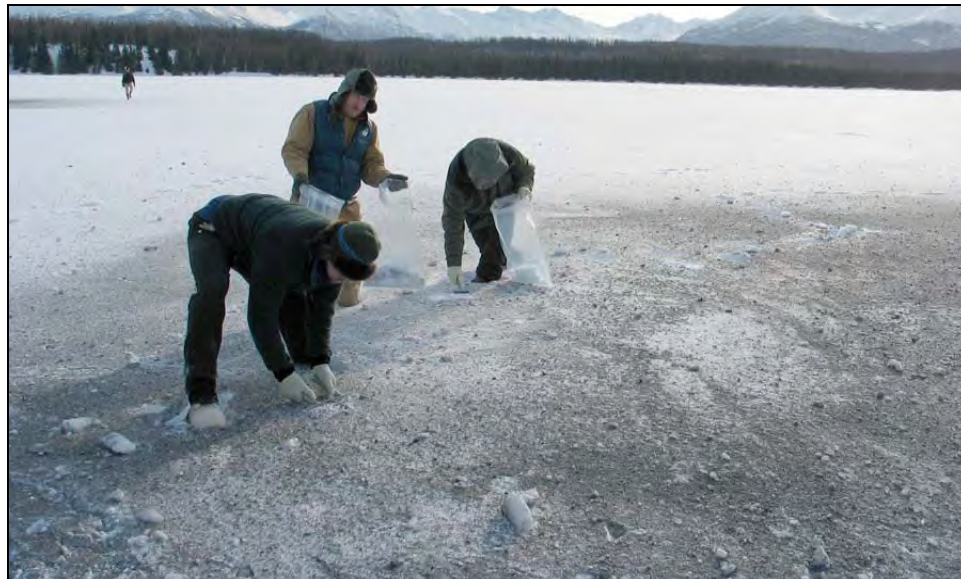
Figure 6. Collecting adjacent MIS samples and subsurface samples from 155-mm plume.
