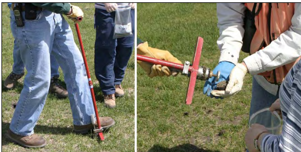
Figure 4. Coring tool designed specifically for collecting multi-increment cohesive soil samples.
