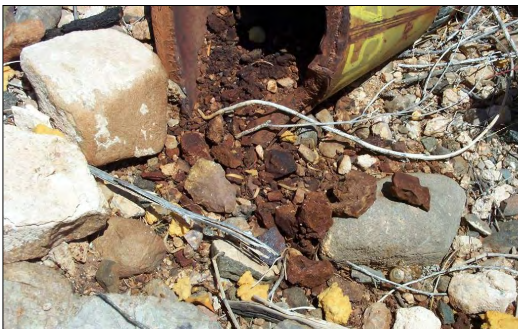
Figure 11. Example of an 155-mm artillery round that has undergone a low-order detonation. Explosive fill is still present in and around the casing.
