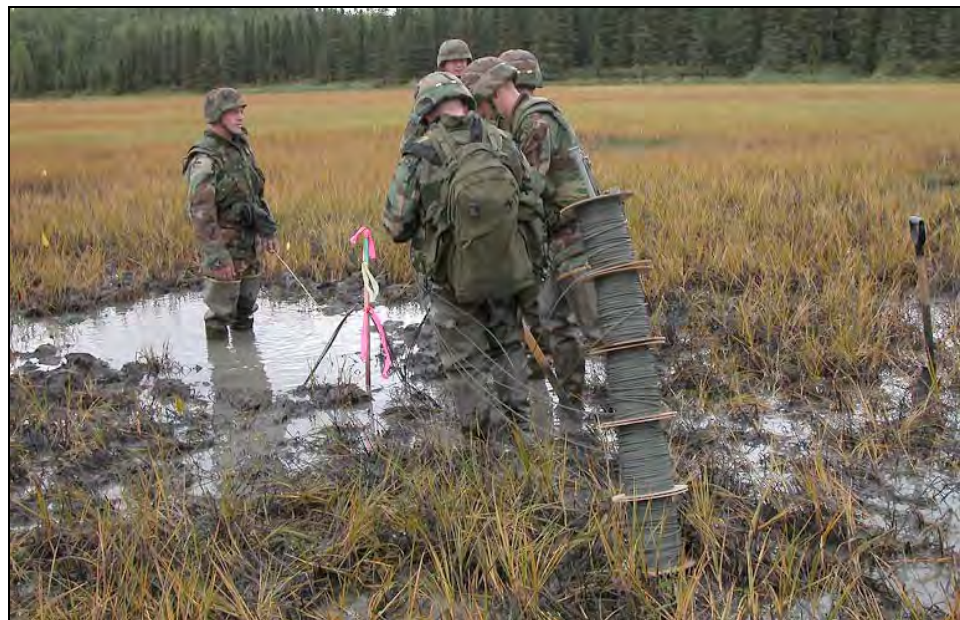
Figure 11. Field assembly of a five-strand det cord run.
