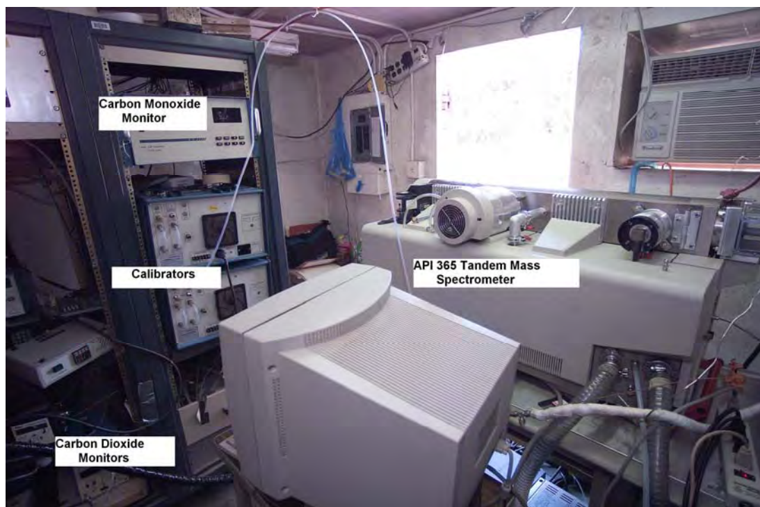
Figure 3.20. Interior View of Bombproof Shelter 2 from Rear. Some Measurement Systems are Noted
