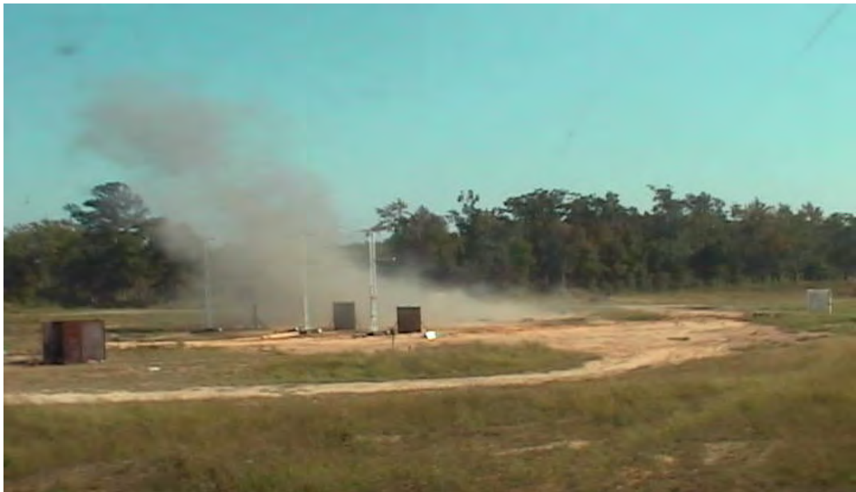
Figure 4.6. Test of 4.2 in. High Explosive Mortar Round. Emissions Cloud is Being Sampled by Tower 1 (left-most tower)
