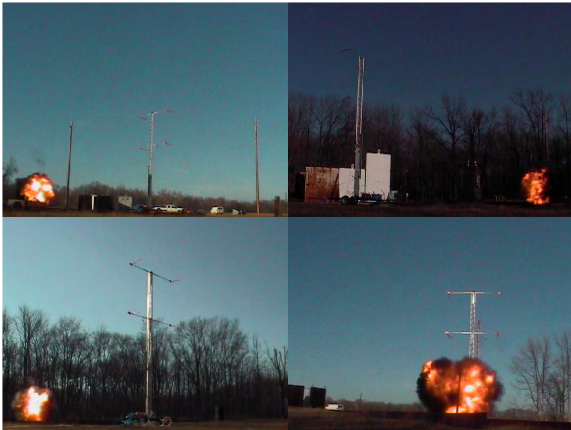
Figure 3.2. Multiple-Angle Views of the Instant of Detonation for a C4 Charge
