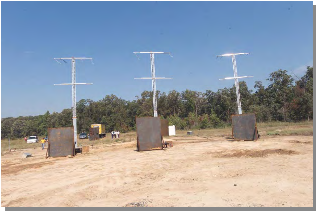
Figure 3.16. POI Sampling Towers with Shields in Place. Photo Taken Near Location of Detonation Point. Bombproof Shelters are Visible in the Background Behind Center Tower. (Note: Vehicles and non-critical personnel were cleared from the range prior to each test.)
