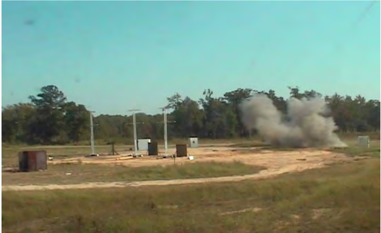
Figure 4.5. Test of 4.2 in. High Explosive Mortar Round Just After Detonation
