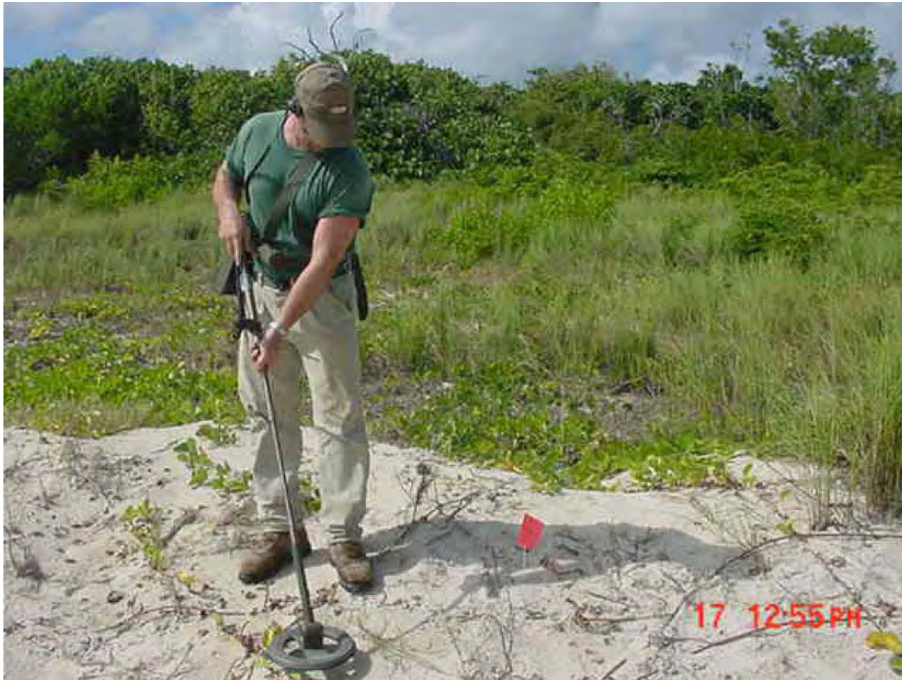
15. Anomaly reacquisition with metal detector.
