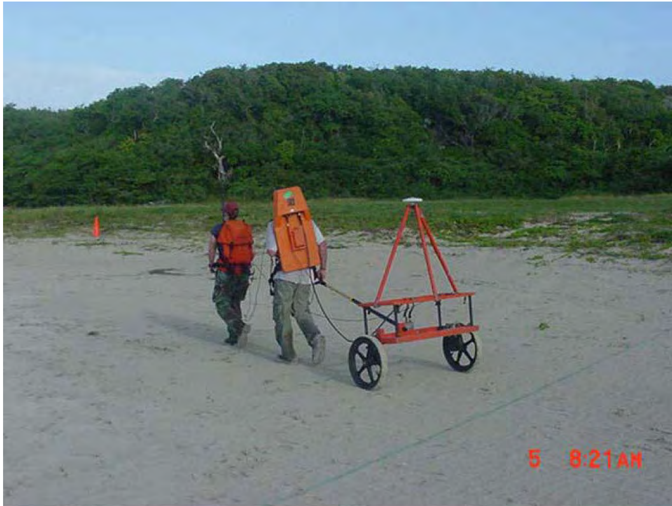
17. Geophysical survey along Red Beach with EM-61 magnetometer and DGPS.
