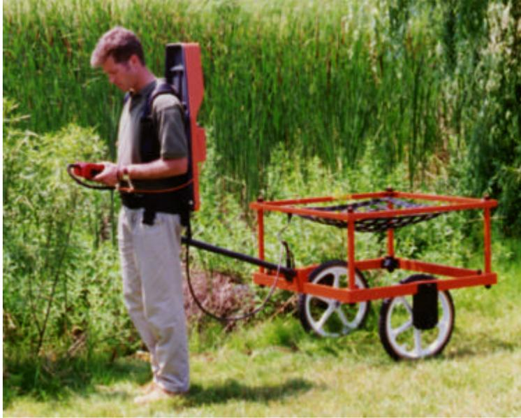
Figure 2-3. Geonics EM61 Magnetometer.
