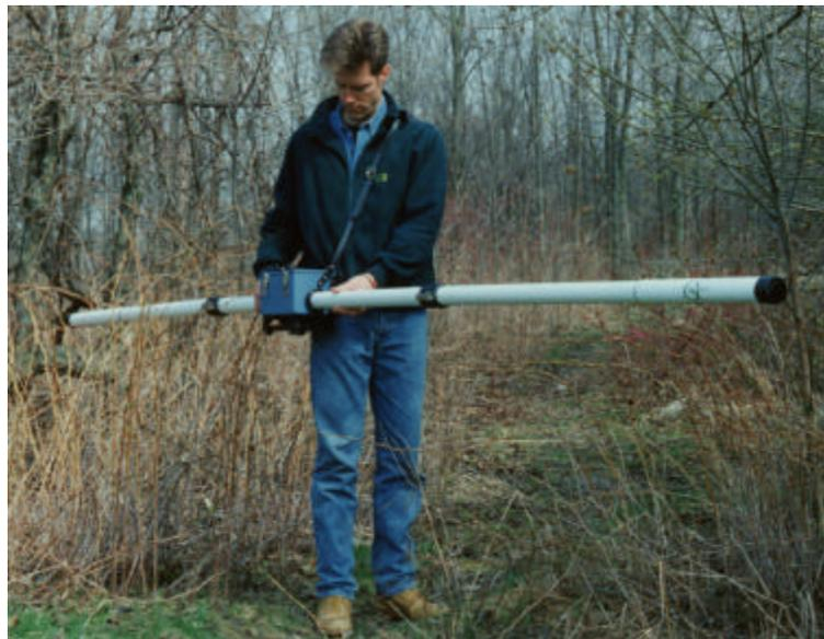
Figure 2-4. Geonics EM31 Magnetometer.
