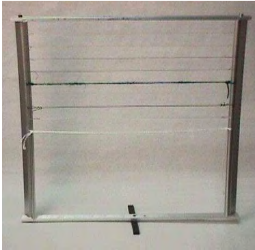
Figure 3. The metal frame with military and improvised tripwires installed.
