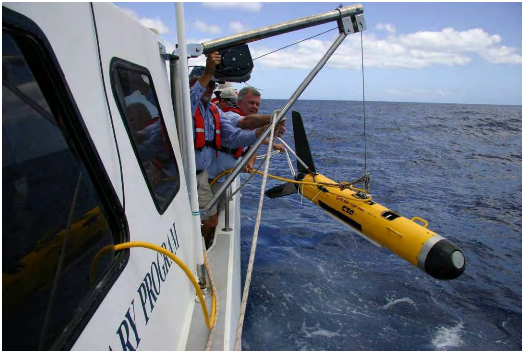
Figure 26. Teledyne Benthos C3D side scan sonar.
