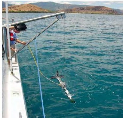
Figure 30. Teledyne Benthos 1624 side scan sonar
