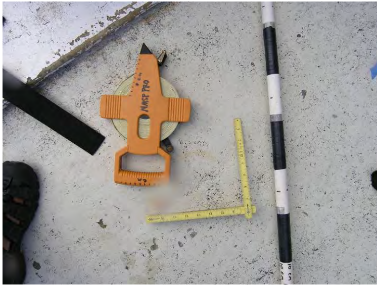
Figure 20. Diver measurement tools (black and white PVC scale used in photos in 10cm sections).
