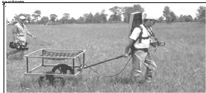
Figure 13. Typical EM Induction System
