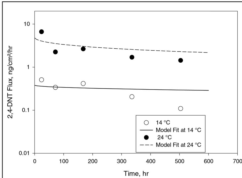
Figure 10. Effect of temperature on the flux of 2,4-DNT from LAAP-C soil (case 2: 20-percent poisture content with dry air passing over the soil)
