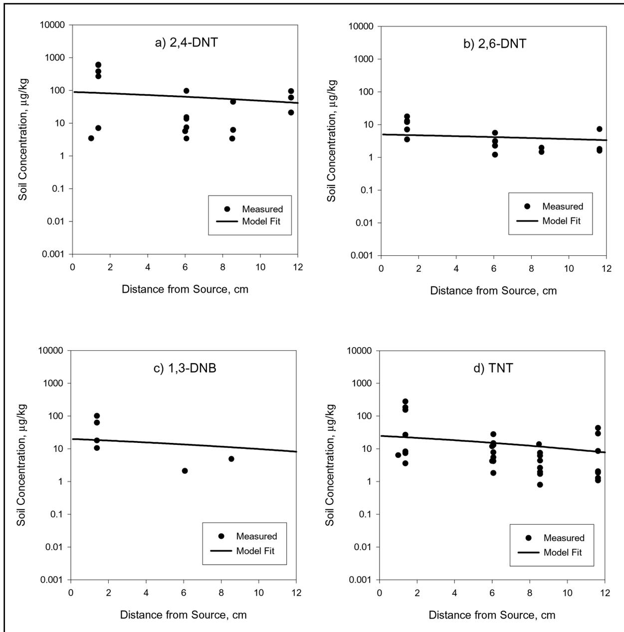
Figure 14. Comparison of experimental (data from Jenkins et al. (2000)) and model fit soil concentrations of 2,4-DNT, 2,6-DNT, 1,3-DNB, and TNT from buried TMA-5 type landmine, Fort Leonard Wood site, 270 days following burial
